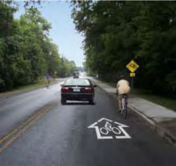
Shared roadways consist of a combined travel lane for motorists and bicyclists.
