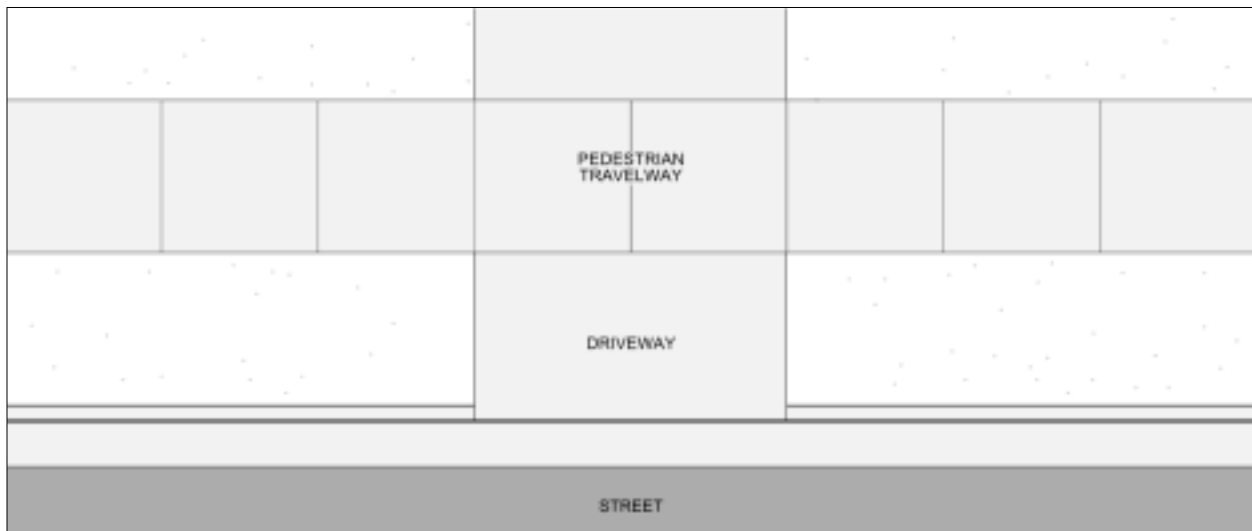
Figure 7: The Pedestrian Travelway shown crosses the driveway without a change in cross slope or scoring pattern, as recommended.
