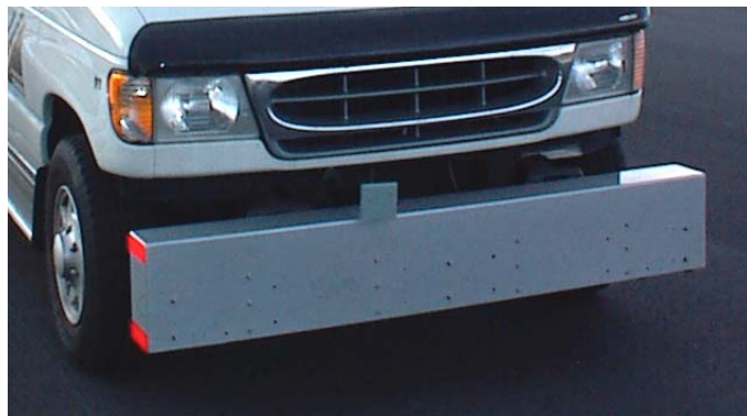
Figure 3.2. Profiler on Digital Survey Vehicle.
